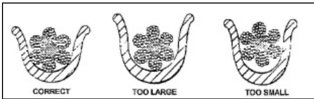
Fig 7-2-1 Correct and incorrect sheaves for a rope
